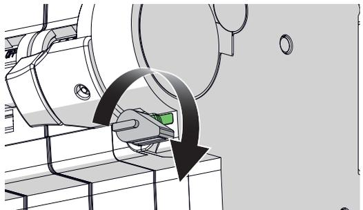
Before manual opening the operator shall disable remote commands through the rotation of activation lever.
