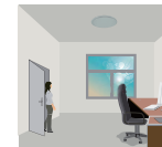
With sufficient natural light, the light does not switch on when presence detected.
