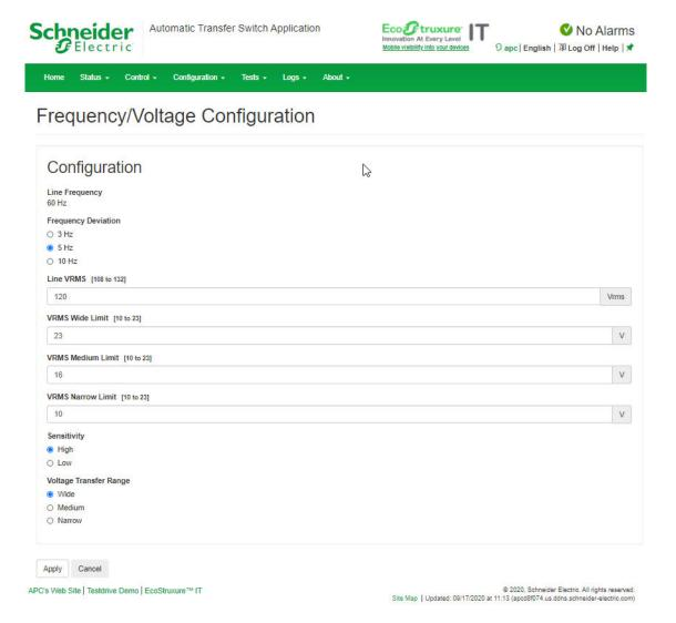
**Frequency Deviation:** Frequency deviation beyond the set value will cause the Rack ATS to switch power sources.
