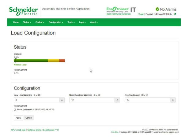
**Status:** View the current in A, and the Peak Current in kVA, for the device, phases, and banks. The indicator in the green, yellow, and red meter shows the load status: normal, near overload, or overload.
