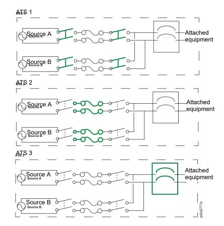
The rack ATS does not include power surge protection. To help protect your ATS from external power surges, it is always recommended that you connect each ATS source to a Double Conversion On-Line Uninterruptible Power Supply (UPS).
