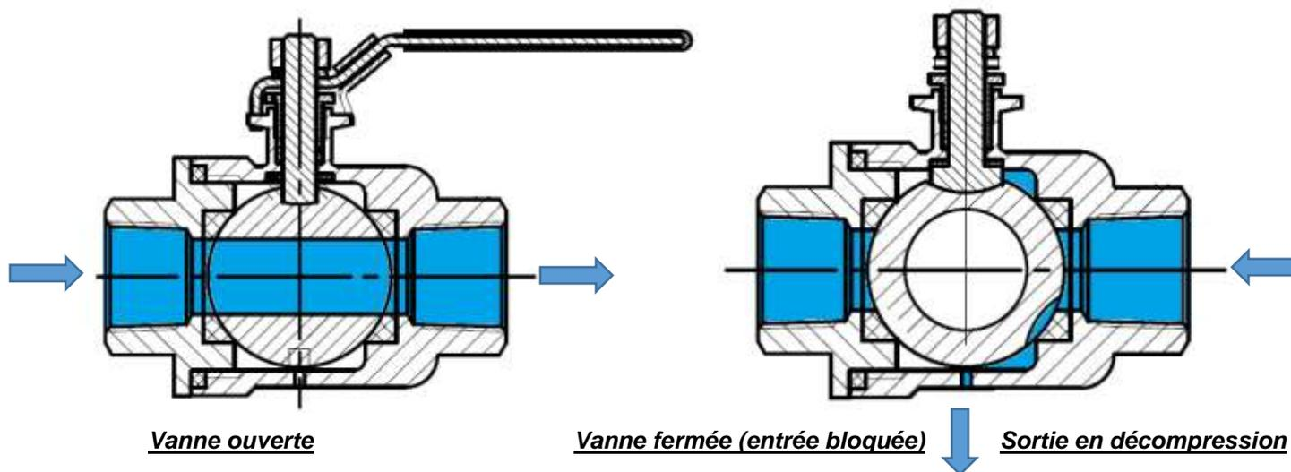
**ROBINET A TOURNANT SPHERIQUE INOX 2 PIECES A DECOMPRESSION BSP**
