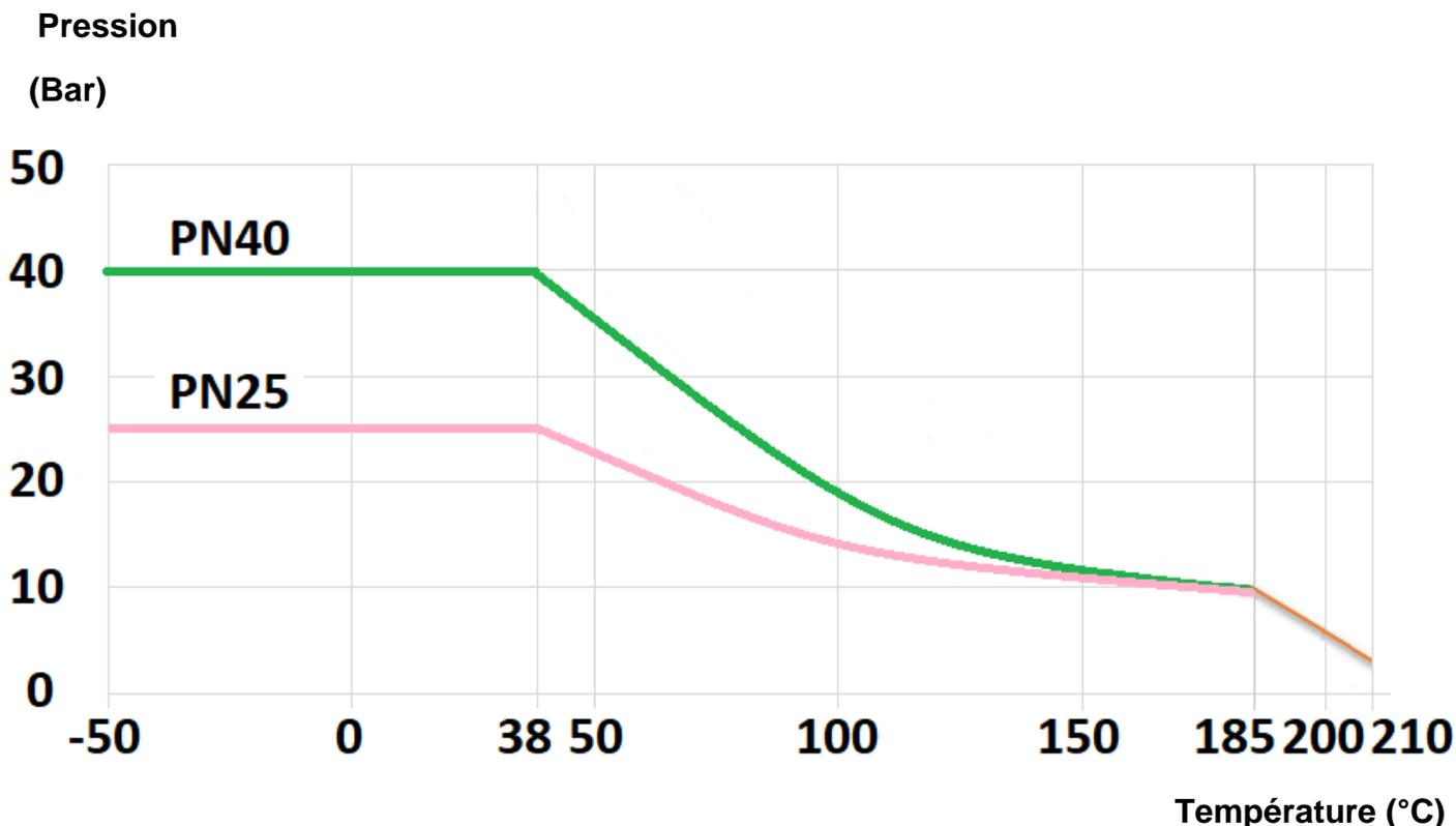
**ROBINET A TOURNANT SPHERIQUE 3 PIECES ELSA DOUBLE BLOCK AND BLEED RF**
