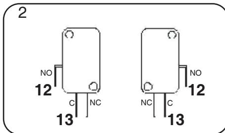
① If there is more than one opening contact, they must be connected in parallel (see picture 2).
