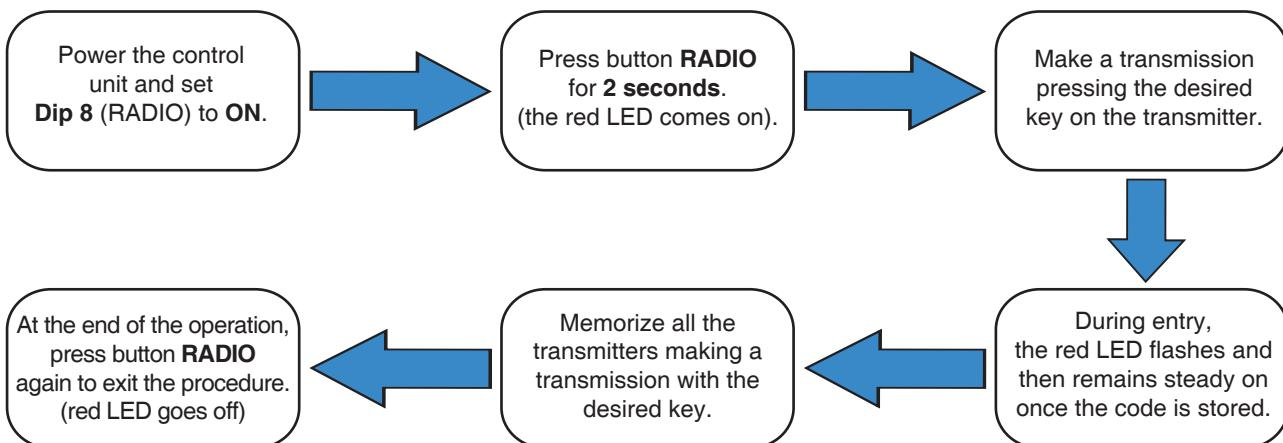
! The programming procedures are exited automatically in any case 10 seconds after the last transmission.
