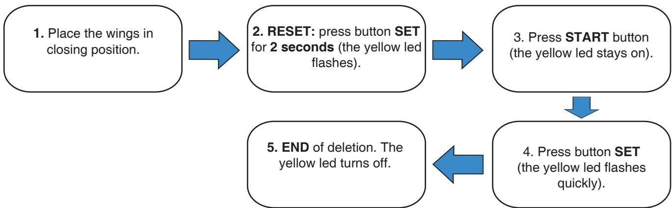
After the deletion, it will be possible to activate the pedestrian opening only by wire, and the size of the opening will be total on the wing opened by MOT1 (terminals 24,25)
