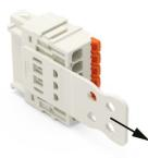
Insert the strain relief plate into the receptacle and pull until it hits the backstop in the conductor connection direction.
