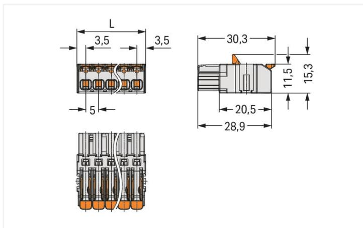
$L = (\text{pole no.} \times \text{pin spacing}) + 2 \text{ mm}$
